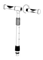
1. Tighten the handle in the direction of the arrow.
